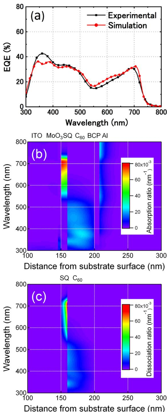
FIG. 2. (a) Experimental and simulated EQE spectra of SQ/C<sub>60</sub> bilayer OPV cells; (b) absorption profile, and (c) exciton distribution for effective charge generation.
