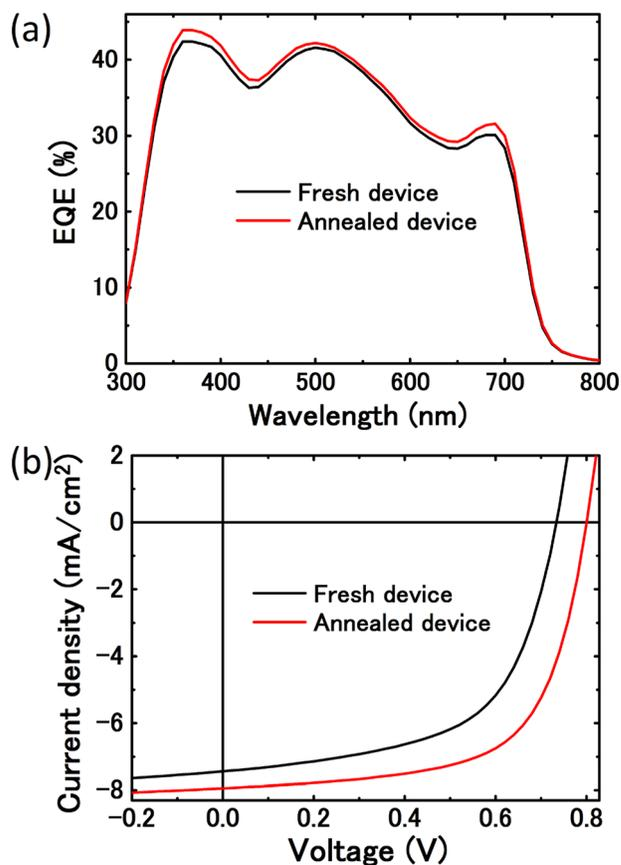
FIG. 3. (a) EQE spectra and (b) J-V characteristics illuminated at 100 mW/cm<sup>2</sup> (AM 1.5 G solar spectrum) for the SQ (9 nm)/C<sub>70</sub> (40 nm) bilayer OPV cells.
