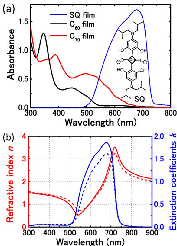
FIG. 1. (a) Molecular structure of SQ, and absorption of SQ, C<sub>60</sub>, and C<sub>70</sub> films (100 nm); (b) optical constants of SQ films on Si substrate. (b) Optical parameters of SQ film,  $n_o$  (red solid),  $n_c$  (red dotted),  $k_o$  (blue solid), and  $k_c$  (blue dotted).
