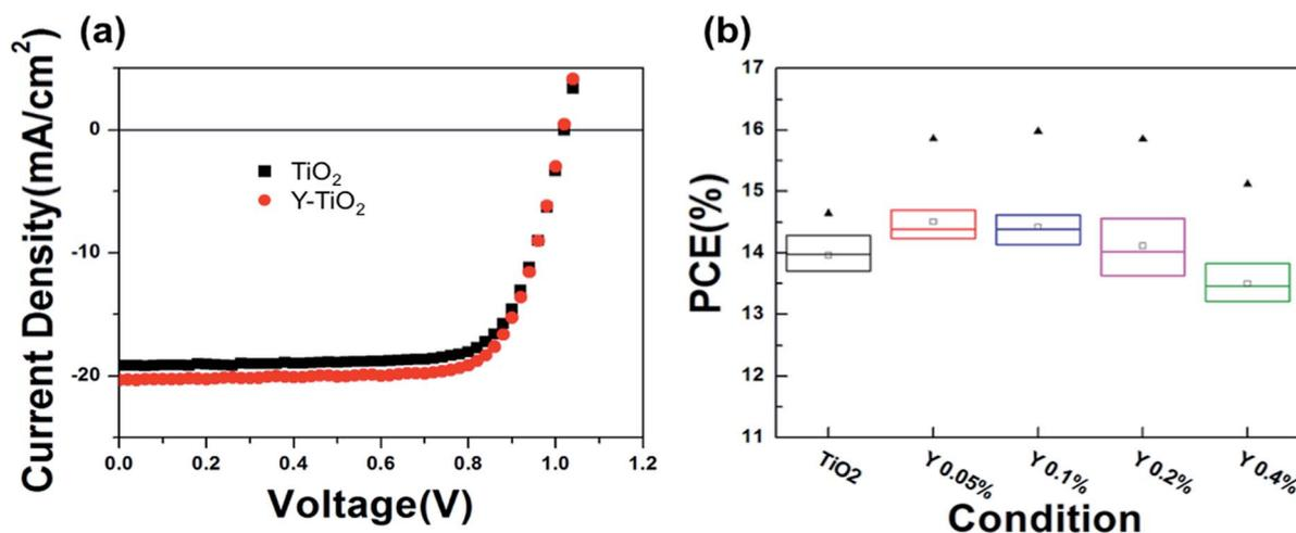
Fig. 1 (a) Typical device  $J$ - $V$  curve of the  $\text{TiO}_2$  ETL incorporated with  $\text{YAC}_3$ . (b) Devices statistics of the PCE based on different concentrations of  $\text{YAC}_3$  incorporated into the  $\text{TiO}_2$  ETL. The three horizontal lines in the box indicate the 25<sup>th</sup>, 50<sup>th</sup> and 75<sup>th</sup> percentile of devices. The triangle and the hollow squares represent the highest and the average value, respectively.
