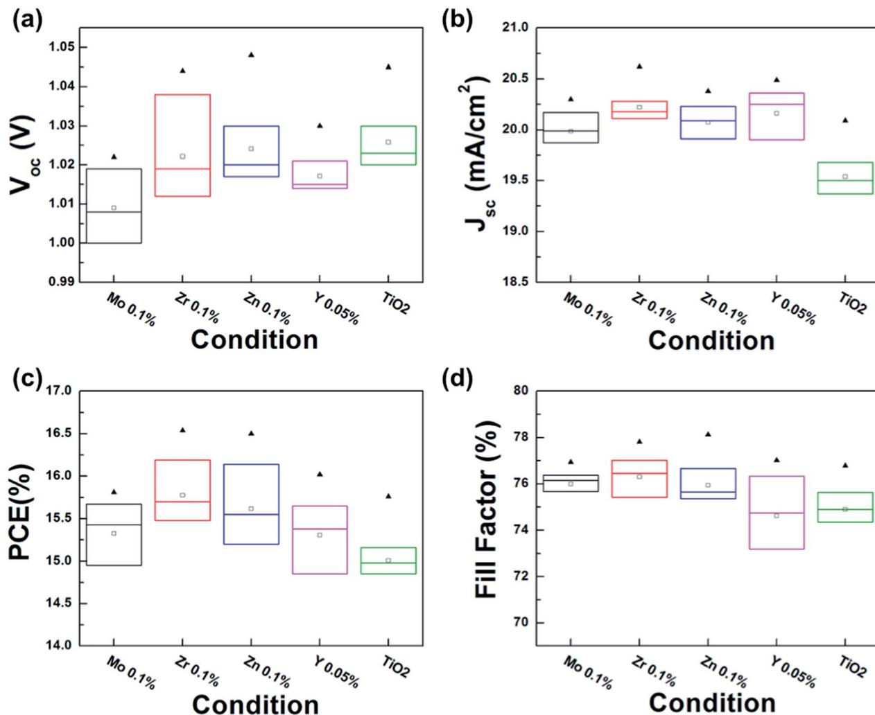
Fig. 3 Device statistics of (a)  $V_{oc}$ , (b)  $J_{sc}$ , (c) PCE and (d) fill factor of the perovskite solar cell employing the ETL incorporated with different acetylacetonate-based additives. The three horizontal lines in the box indicate the 25<sup>th</sup>, 50<sup>th</sup> and 75<sup>th</sup> percentile of devices. The triangle and the hollow squares represent the highest and the average value, respectively.
