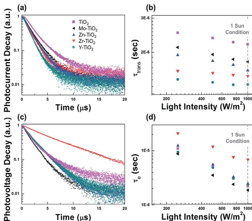
Fig. 4 Photocurrent and photovoltage decay of devices employing the TiO<sub>2</sub> ETL incorporated with different acetylacetonate-based additives and the related carrier transport lifetime and electron lifetime. Intensity is shown in log scale and 1 sun condition is equivalent to 1000 W m<sup>-2</sup>.
