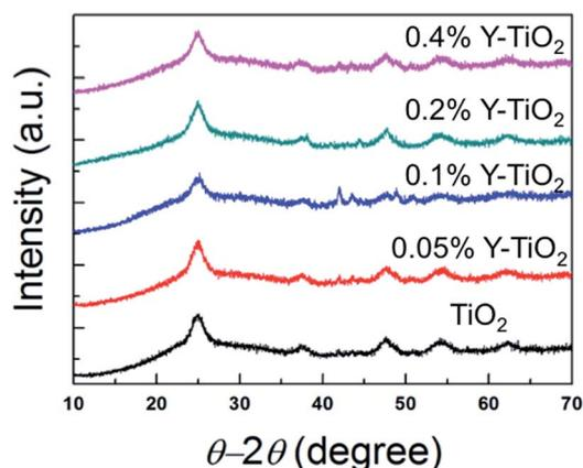
**Fig. 2** X-ray  $\theta$ - $2\theta$  scan of the TiO<sub>2</sub> ETL incorporated with different concentrations of  $\text{YAc}_3$ .
