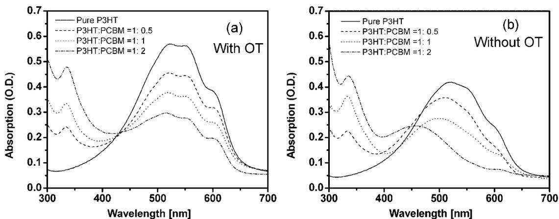
**Figure 2.** Absorption of P3HT:PCBM composite layer of pure P3HT (solid line), P3HT:PCBM weight ratio 1:0.5 (dashed line), 1:1 (dotted line), and 1:2 (dashed-dotted line) processed with (a) and without (b) 1,8-octanedithiol in the blend solution.
