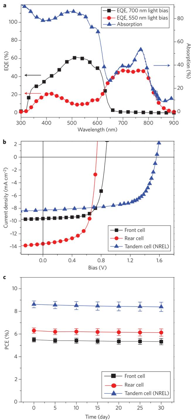
**Figure 4 | Quantum efficiencies, *J*-*V* characteristics and stability of single cells and tandem cells. **a**, EQEs of the inverted tandem solar cell and absorption spectrum (without metal electrode). **b**, *J*-*V* characteristics of the front cell, rear cell and inverted tandem solar cell, tested at NREL using the OSMSS simulator. **c**, Stability of the inverted front cells, rear cells and tandem cells (tested at UCLA).**
