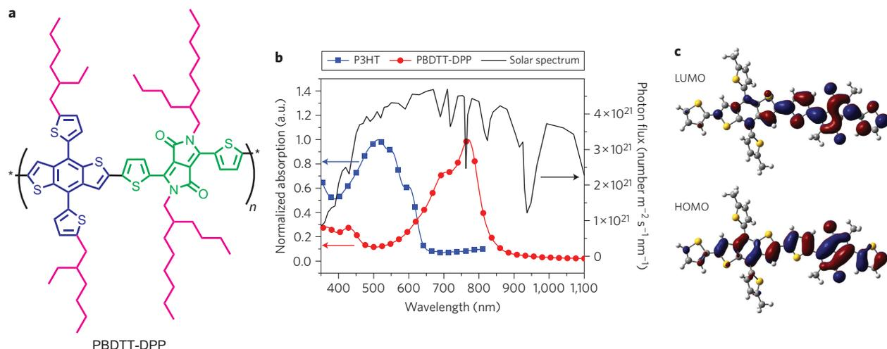
**Figure 1 | Molecular design, optical properties and electron density of HOMO and LUMO for PBDTT-DPP.** **a**, Chemical structure of PBDTT-DPP. **b**, UV-visible absorption spectra of PBDTT-DPP and P3HT films and the solar radiation spectrum. The UV-visible absorption profiles of PBDTT-DPP and P3HT show that the two materials cover the solar spectrum from 350 to 850 nm in a complementary manner. **c**, Electron density of HOMO and LUMO for PBDTT-DPP computed by density functional theory (DFT).
