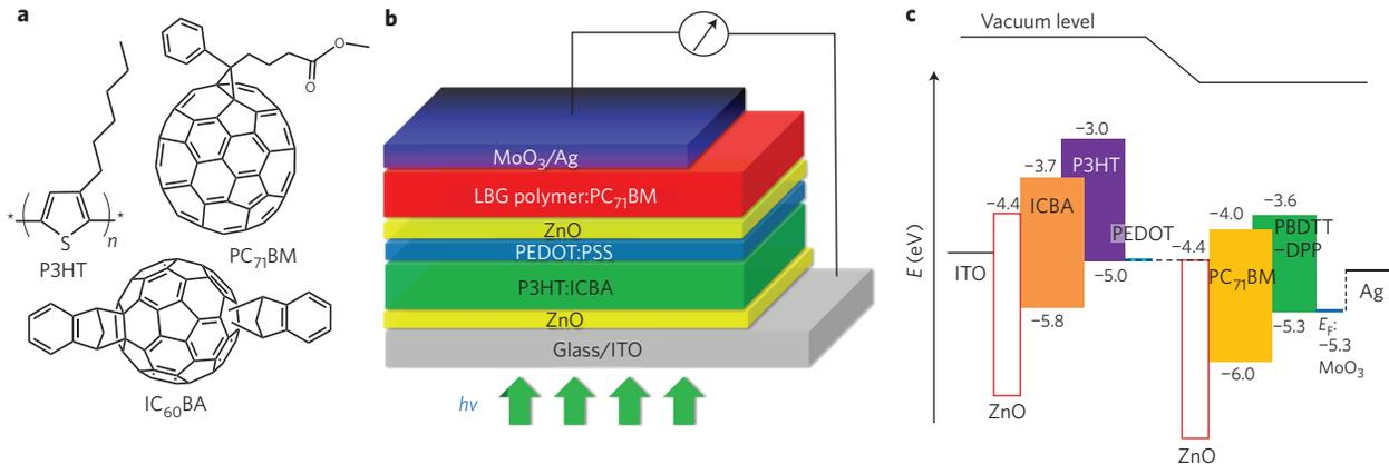
**Figure 3 | Inverted tandem solar cells.** **a**, Chemical structures of P3HT,  $\text{IC}_{60}\text{BA}$  and  $\text{PC}_{71}\text{BM}$ . **b**, Device structure of the inverted tandem solar cell (LBG, low bandgap). **c**, Energy diagram of the inverted tandem devices.
