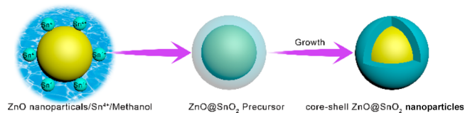
Figure 1. Synthetic diagram of core–shell ZnO@SnO 2 nanoparticles.
