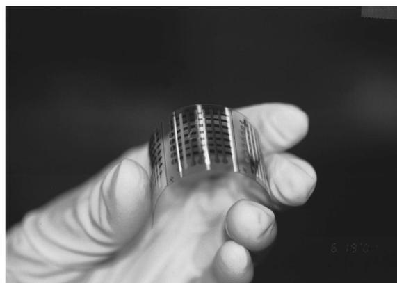
FIG. 3. Photograph of  $7 \times 7$  organic memory array on a regular plastic overhead transparency.
